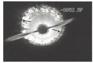
Photo 031 Joint in 85/8" slotted pipe
